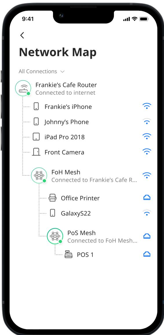
The Network Map provides a topological view of your network. To view the Network Map, tap **Networks** on the dashboard. Next, tap **Network Map** to view devices connected to your system.
